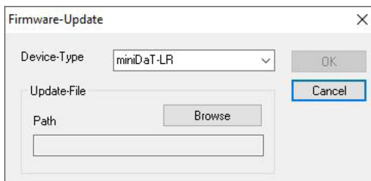
Then choose the type of device for the DaT device, which should be updated, and via the button „Browse“ set the path to the Firmware-Update, which you have received from the Rösler company.
