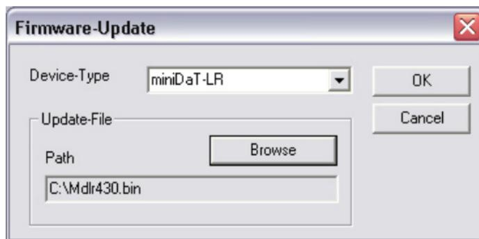
Confirm with „OK“ your selection of the device resp. file. In the following menu you set the interface, which you want to use for data transfer, and the device, that should be updated. Here in our example we update a miniDaT-LR, therefore we must select the setting „Local Radio“ for the port (in this case we must connect a miniDaT-IAP to the port). If the device isn't shown in your range „Internal No“, data transfer number has to be entered manually.
