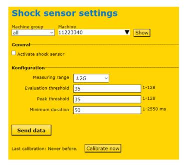
After installing the device, the acceleration sensor should be calibrated.
