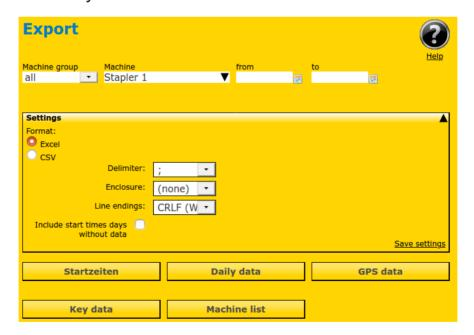
With the export function, start times, daily data, GPS data, key data and machine list of a machine can be exported.
