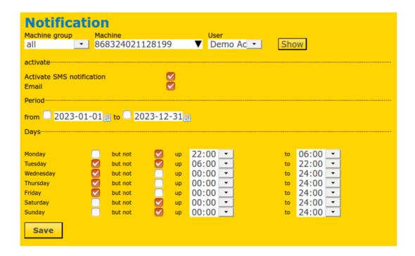
The alarm messages will be sent from the server to all users activated for the device via SMS and/or e-mail. It is important that a valid mobile telephone number and/or e-mail address is entered for the respective user in the master data. After sending an alarm message, monitoring for the device will be disabled to prevent repeated SMS/e-mails.
