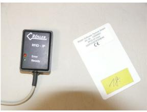
reaction of safety equipment. These parameters form on the one hand the basis for the corresponding invoicing. On the other, however, in the event of damage it is possible to definitely trace who caused it. Two products from Rösler Software-Technik are used here: firstly, Rösler Access, i.e. electronic access control, done here using a card reader and a correspondingly programmed card. Secondly, the Rösler Obserwando system, i.e. the web-based service, with which you have direct contact
